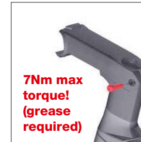
Install stem steerer clamp bolt - grease required!
